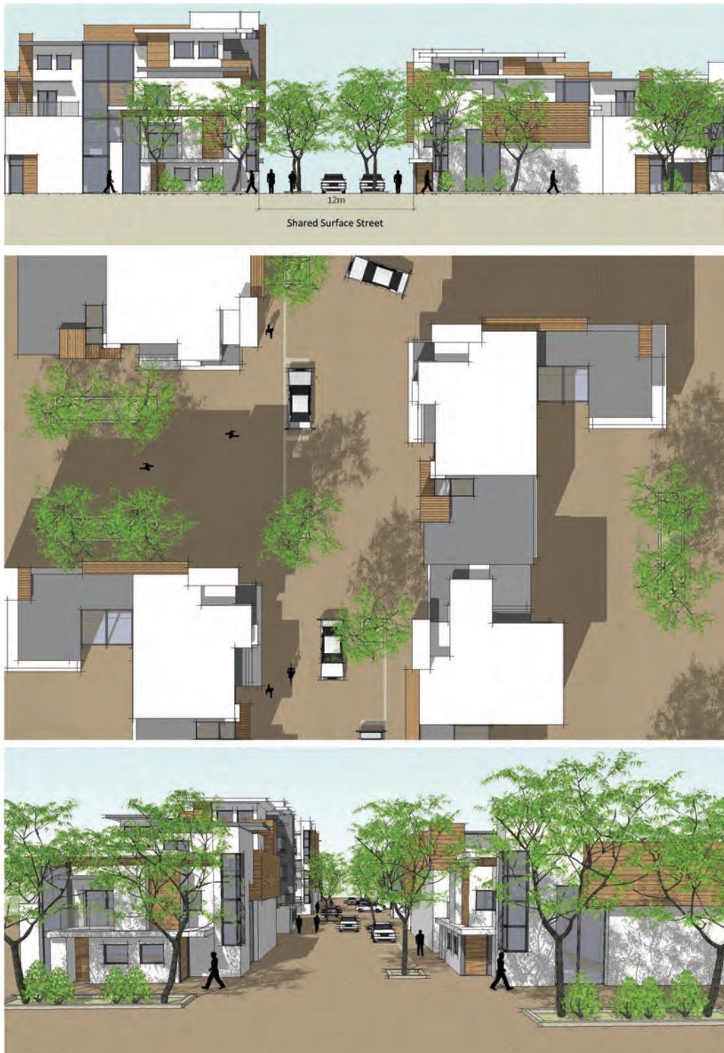
Figure 14.17: Shared Surface Street
